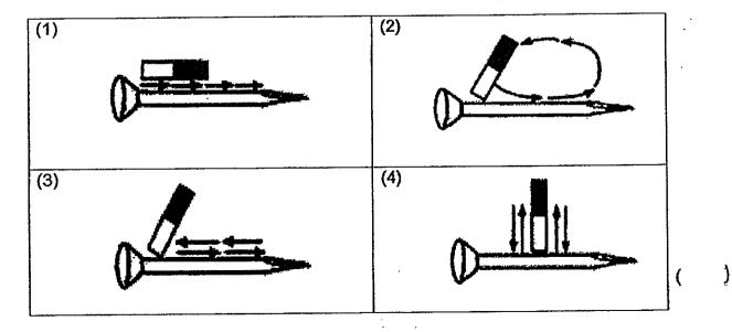
20. Jie Min learnt that an iron nail is magnetised when it is wound with a coil of wire connected to batteries.
