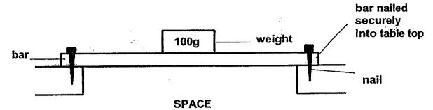
He placed 100g weights one by one on the materials until the bar broke.
