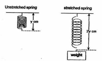
Upon removing the mass, the spring returns to its original length, y cm. Next, if a mass twice as heavy as the original mass was hung from its end, what will be the new length of the spring?
