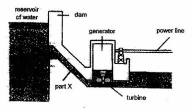
What are the advantages of storing a large quantity of water in the dam and controlling the flow of water over the turbines?
