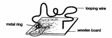
Sammy must not allow the metal ring to touch the looping wire as he moves the ring through the wire from the start to the end of the loop. Otherwise, the buzzer will sound instantly and he will have to begin all over again.
