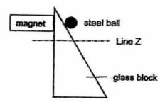
The magnet was slid down the vertical side of the triangular glass block at a constant speed. It was observed that the steel ball also slid down in tandem on the other side of the glass block until it passed Line Z where it rolled down the block.
