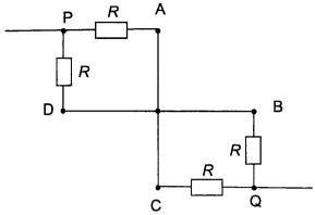
The effective resistance between P and Q is the twice of the net resistance of two resistors (across points P & D and P & A) in parallel. The effective resistance between P and Q = R.
