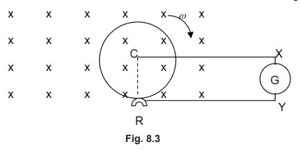
Between C and R, there would be an induced e.m.f., which may be indicated by a galvanometer connected between X and Y  $\,$
