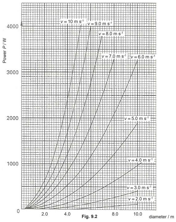
Fig. 9.2 shows how P, the output power of these windmills, varies with the overall diameter of the wheel for different wind speeds, v.
