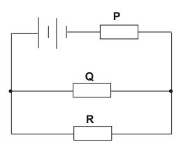
The battery, of negligible internal resistance, supplies a total power of 12 W. What is the power dissipated in resistor **R**?
