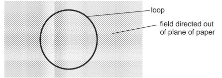
The field is directed out of the plane of paper. The magnitude of the magnetic flux density is decreasing at a constant rate.
