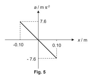
(a) (i) Show that the angular frequency of the vertical oscillation is 8.7 rad s<sup>-1</sup>. [2]
