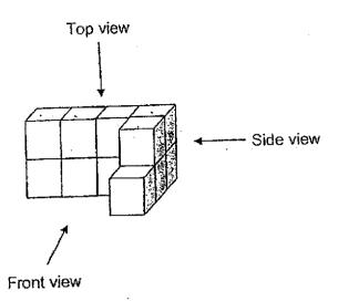
Draw the front view and the top view of the solid on the grids below.
