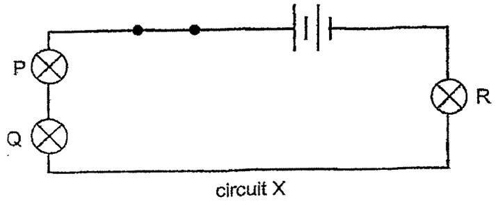
(a) Based on circuit X, explain why it is not safe to ride the scooter at night if lamp Q fuses. [1]
