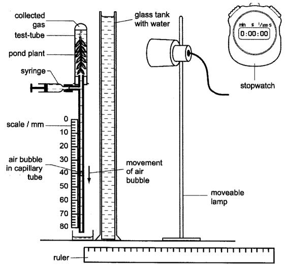
The student maintained the temperature at 25 °C and measured the distance travelled by the air bubble in the capillary tube for a period of five minutes for each light intensity.
