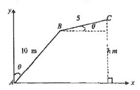
The diagram shows an extended mobile crane made up of a movable boom AB and a movable jib BC. At a certain time, the crane is in a vertical plane. Ax is horizontal and Ay is vertical. The boom makes an angle of  $\theta$  with the vertical and the jib makes an angle of  $\theta$  with the horizontal. The lengths of AB and BC are 10 in and 5 m respectively. Given that C is h in above Ax,
