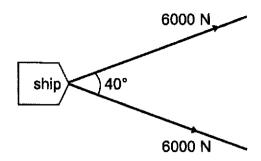
(a) The angle between the forces exerted by the two tugs is 40°. Each tug pulls with a force of 6000 N. Draw a scale diagram to determine the resultant force that the tugs exert on the ship.
