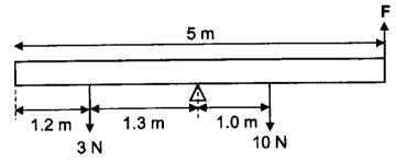
What is the magnitude of upward force F needed to keep the beam horizontal?
